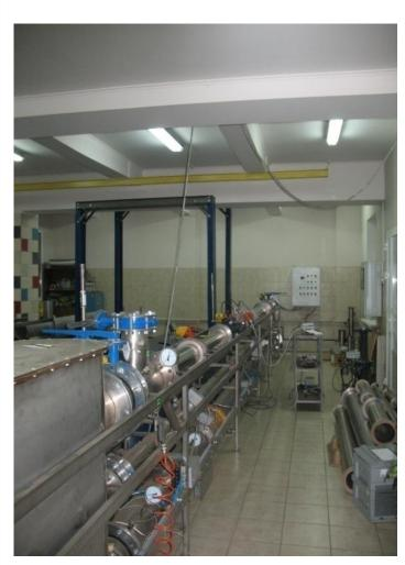
Automated proving rig APU-G-011/5000 is intended for calibration and proving flow meters working on air, natural gas, and other gases and mixtures.
